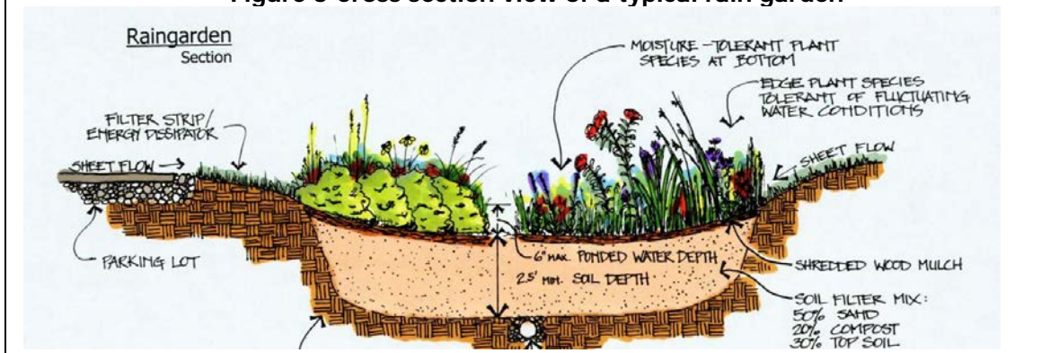
Figure 5 Cross section view of a typical rain garden
